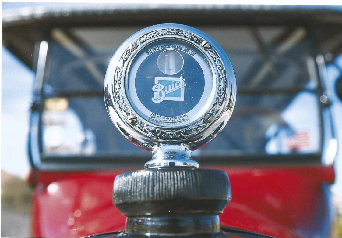
The Buick's hood ornament is original and also serves as the car's radiator cap and temperature gauge (a thermometer is built in). STEVE CRAFT FOR THE WALL STREET JOURNAL
